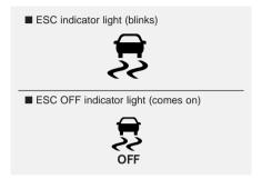
When the POWER button is pressed to the ON position, the ESC indicator light illuminates, then goes off if the ESC system is operating normally.
