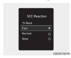
The sensitivity of vehicle speed when following the front vehicle to maintain the set distance can be adjusted. Go to the 'User Settings → Driver Assistance → SCC Reaction → Fast/Normal/Slow' on the LCD display. You may select one of the three stages you prefer.
