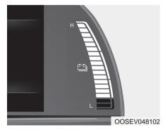
The SOC gauge shows the charging status of the high voltage battery.
