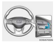
Push the switch (1) up (RES+). If the vehicle speed is over 20 mph (30 km/h), the vehicle will resume the preset speed.
