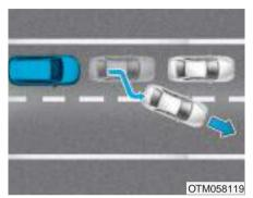
When driving in stop-and-go traffic, and a vehicle in front of you merges out of the lane, the FCA system may not immediately detect the new vehicle that is now in front of you. In this case, you must maintain a safe braking distance, and if necessary, depress the brake pedal to reduce your driving speed in order to maintain a safe distance.
