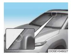
Auto defogging helps reduce the possibility of fogging up the inside of the windshield by automatically sensing the moisture on inside the windshield.
