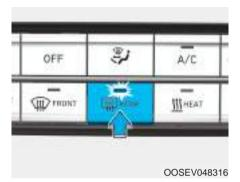
The defroster heats the window to remove frost, fog and thin ice from the interior and exterior of the rear window, while the vehicle is in the ready ( ) mode.
