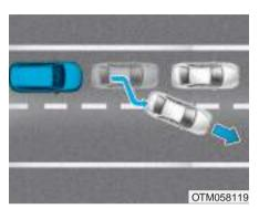
When driving in stop-and-go traffic, and a vehicle in front of you merges out of the lane, the system may not immediately detect the new vehicle that is now in front of you. In this case, you must maintain a safe braking distance, and if necessary, depress the brake pedal to reduce your driving speed in order to maintain a safe distance.
