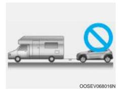
Your vehicle is not designed to be flat-towed behind a motor home. To avoid serious damage to your vehicle, do not flat-tow your vehicle.
