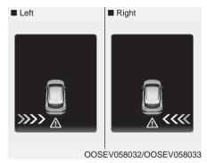
If the vehicle detected by the sensors approaches your vehicle, the warning chime will sound, the warning light on the outer side view mirror will blink and a message will appear on the LCD display.
