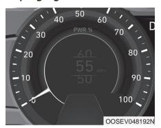
The torque gauge shows the realtime torque value while driving when SPORT mode is selected by pressing the DRIVE MODE button.
