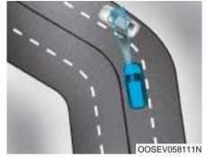
Forward Collision-Avoidance Assist system may recognize a vehicle in the next lane or outside the lane when driving on a curved road.
