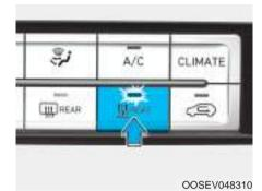
Push the HEAT button to turn the heater on (indicator light will illuminate).
