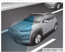
Lane Keeping Assist system helps detect lane markers on the road with a camera at the front windshield, and assists the driver's steering to help keep the vehicle between lanes. When the system detects the vehicle straying from its lane, it alerts the driver with a visual and audible warning, while applying a slight countersteering torque, to try to prevent the vehicle from moving out of its lane.
