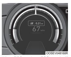
When ECO mode or ECO+ mode (if equipped) is enabled, the speedometer display includes an additional range value which is accumulated as a result of regenerative braking. The value starts from zero and incrementally increases as the energy from regen braking increases. The display resets to zero when the regen level drops to zero (vehicle accelerating, etc.).
