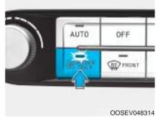
If you press the DRIVER ONLY (\$\mathbb{G}^{\text{DRIVER}})\$ button, the indicator light will illuminate. In this mode the climate control system blows air primarily through the two left-most vents (nearest the driver).
