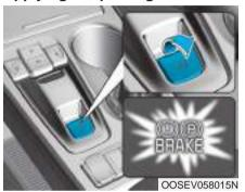
To apply the EPB (Electronic Parking Brake):
