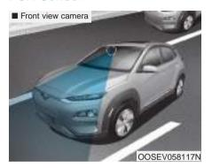
In order for the FCA system to operate properly, always make sure the camera is clean and free of dirt, snow, and debris. Dirt, snow, or foreign substances on the surface may adversely affect the sensing performance of the sensor.
