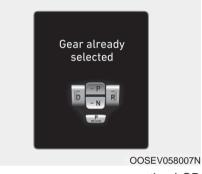
The message appears on the LCD display when the selected gear button is pressed again.
