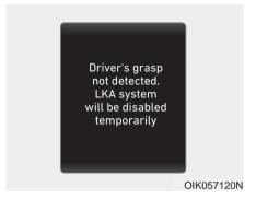
If the driver still does not have their hands on the steering wheel after the message "Keep hands on steering wheel", the system will not control the steering wheel and warn the driver only when the driver crosses the lane markers.
