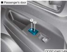
The driver side and front passenger side door armrest is equipped with a central door lock switch.
